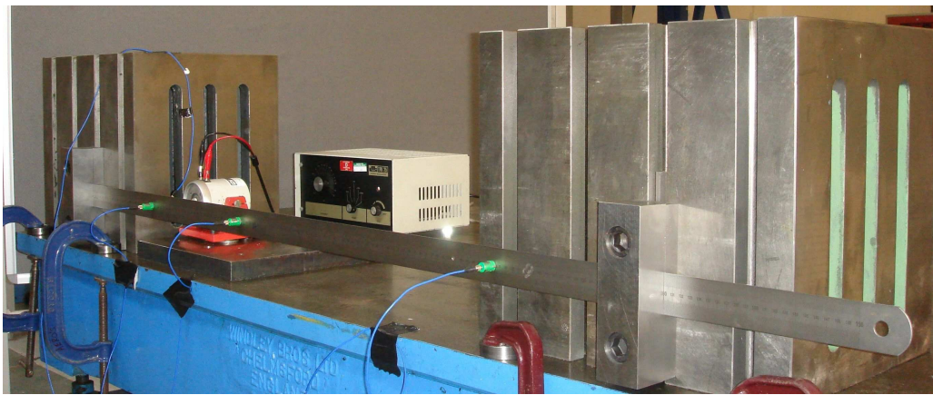
Figure 1. The test rig for the fixed-fixed beam.
