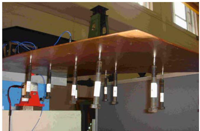
(b) Attached oscillators at random locations. The spring stiffness varies so that the oscillator frequencies are between 43 and 70 Hz.
