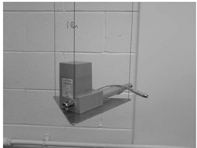
Fig. 3 The actuator in situ on the trifilar suspension plate
