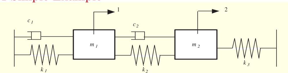
We consider a simple two-degrees-of-freedom system to illustrate the matrix variate distributions. The mean of the mass, damping and stiffness matrices are given by
