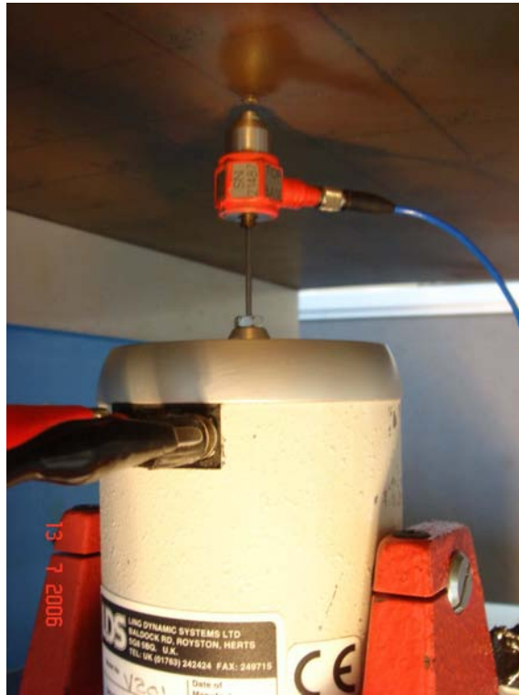
Fig. 6. The shaker used to provide an impulse excitation using a Simulink TM and dSpace TM . A hard steel tip was used and the shaker was placed at node (4,6).
