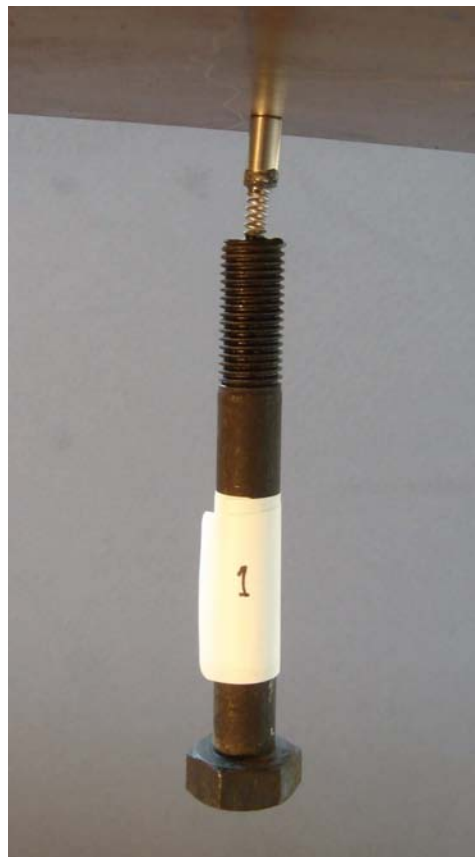
Fig. 3. Details of a typical oscillator used to simulate unmodelled dynamics. Fixed mass (magnet) 2g, oscillatory mass (the nut) 121.4g. The oscillatory mass is about 1% of the total mass of the plate. The spring stiffness varies between 1.5 and 2.4 \times 10^4 N/m.
