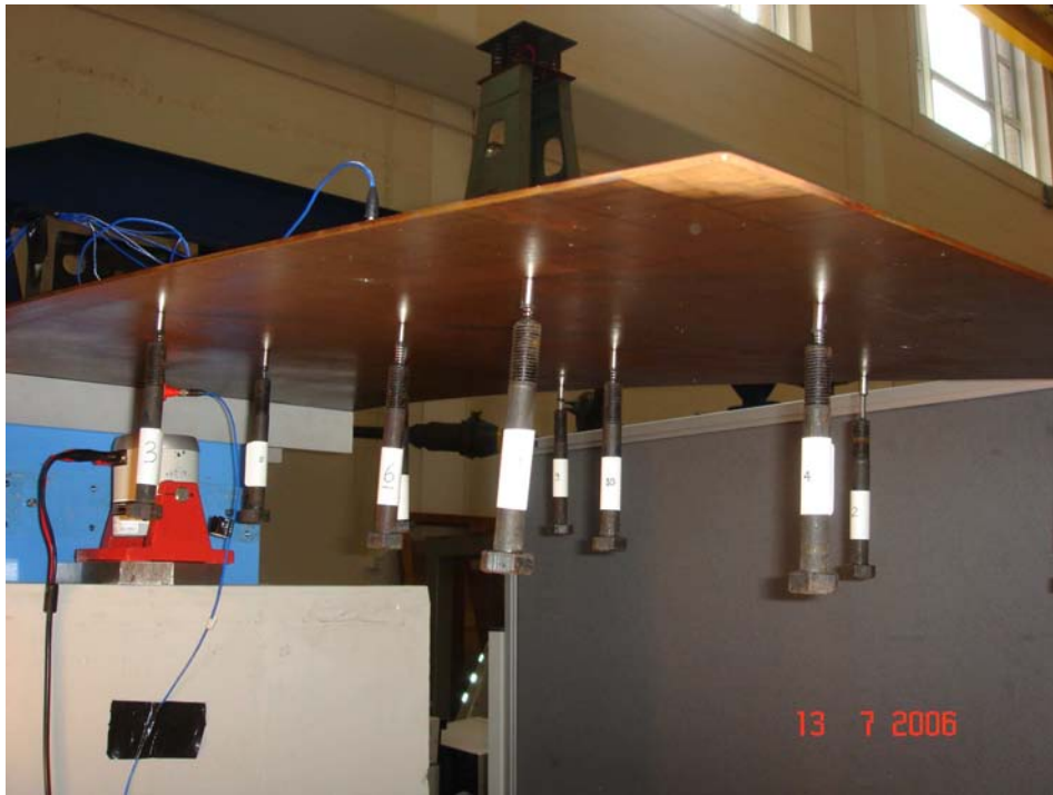
Fig. 4. Attached oscillators at random locations. The spring stiffness varies so that the oscillator frequencies are between 43 and 70 Hz.
