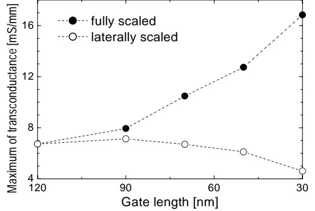
Figure 6: Maxima of transconductance as a function of the device gate lengths for fully scaled PHEMTs compared with those of laterally only scaled devices.
