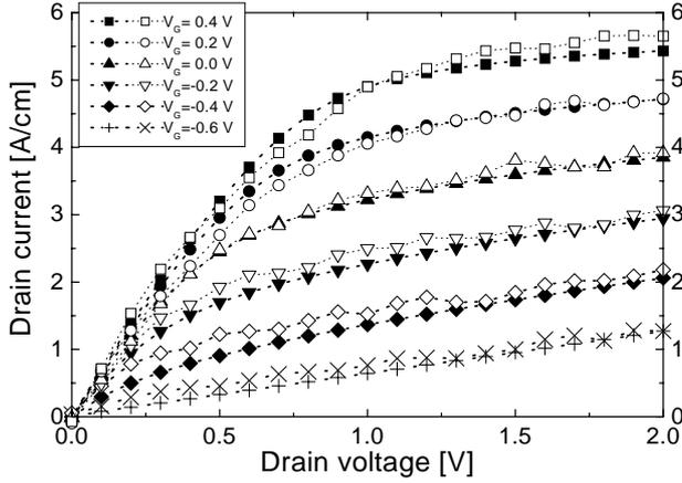
Figure 5:  $I_D$ - $V_D$  characteristic of the PHEMT with a gate length of 120 nm. Full symbols represent experimental data for several fixed gate voltages. Open symbols are MC simulations when external resistances of the drain and source are included.
