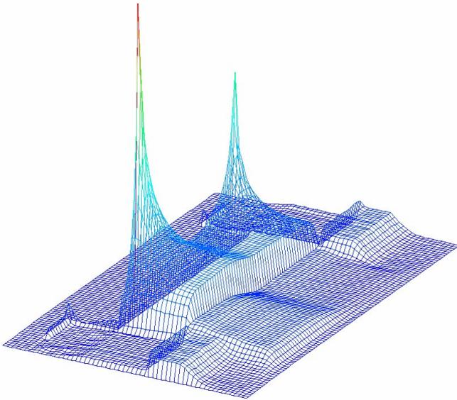
Figure 3: Electric field in the 120-nm gate length PHEMT at  $V_G = -1.0$  V and  $V_D = 2.0$  V. The huge electric fields which surround the gate and peak beneath the recesses determine a particle trajectory after tunnelling.
