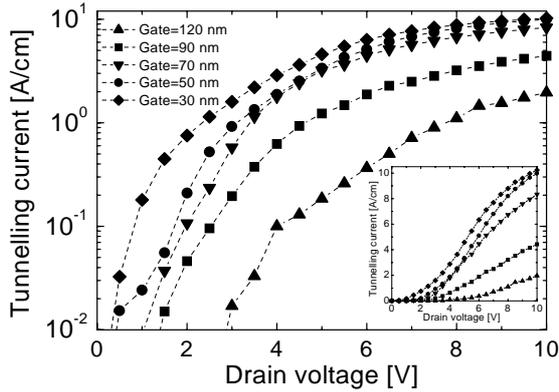
Figure 8: Tunnelling assisted drain current versus the drain voltage at  $V_G = -1.0$  V for the scaled PHEMTs. The inset shows again the same curves on a linear scale.
