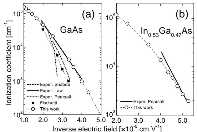
Figure 1: Impact ionisation coefficients versus inverse applied electric field obtained from simulations for GaAs (a) and for In<sub>0.53</sub>Ga<sub>0.47</sub>GaAs (b) compared to experiments and full band simulations.
