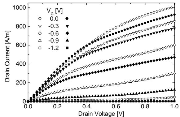
**Figure 4** -  $I_d-V_d$  comparison for 120nm standard (transparent) and self-aligned devices (opaque)
