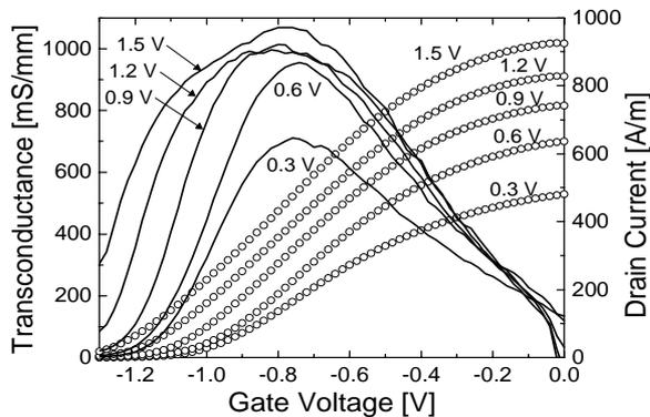
**Figure 6** -  $I_d$ - $V_g$  (circles) and transconductance (full lines) for a 120nm *standard* device. Drain voltages indicated for each sweep.
