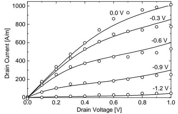
**Figure 7** - Calibration of  $I_d$ - $V_d$  characteristics obtained from MC device simulations (circles) against experimental data (full lines) for a standard 120nm device. Gate voltages are indicated for each sweep.
