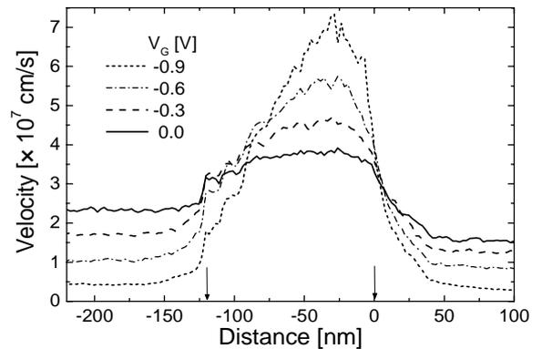
**Figure 8** - Average velocity along the channel for a standard 120nm device at  $V_d = 1.0\text{V}$ . Gate voltages as indicated. The gate region is marked by arrows.
