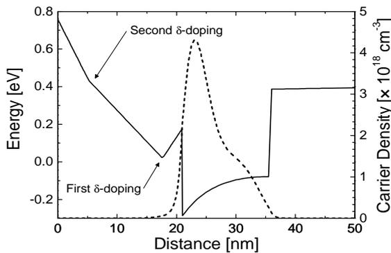
**Figure 2** - Conduction band and carrier concentration profiles vs distance under the gate at  $V_g=0\text{V}$
