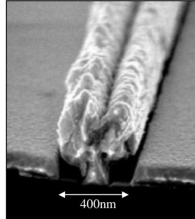
**Figure 3** - SEM image of a self-aligned 120nm T-gate.
