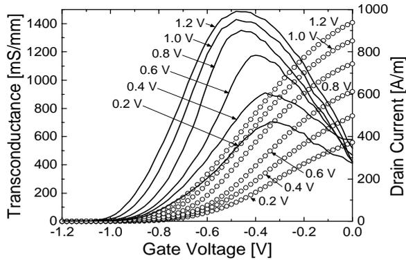
**Figure 5** -  $I_d$ - $V_g$  (circles) and transconductance (full lines) for a 120nm *self-aligned* device. Drain voltages indicated for each sweep.
