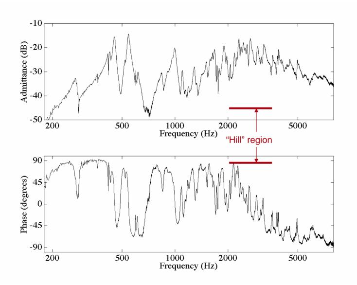
One possible reason for this feature lies in the behaviour of the bridge. A normal bridge has its first in-plane resonance around 3 kHz when the feet are clamped. The mode shape is roughly like this:
