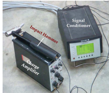
Figure A.1: Impulse hammer, Signal Conditioner and Charge amplifier
