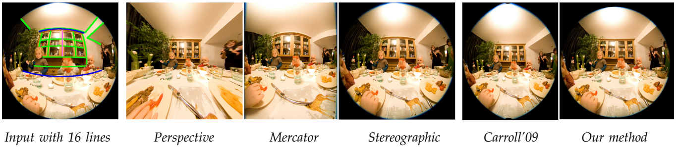
Fig. 6. Output of various still fisheye photograph correction methods.
