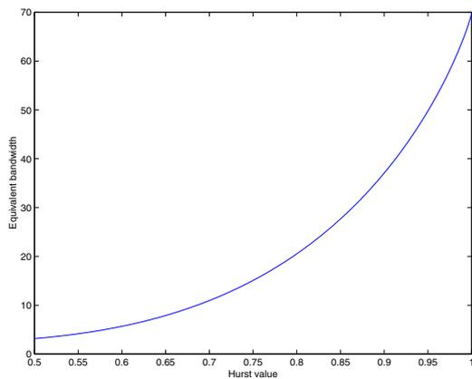
Fig. 8. Relationship between Hurst parameter and equivalent bandwidth
