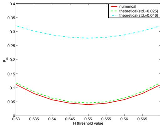
Fig. 3. Misclassification Probability  $P_m$  for  $H = 0.5, 0.6$  traffic
